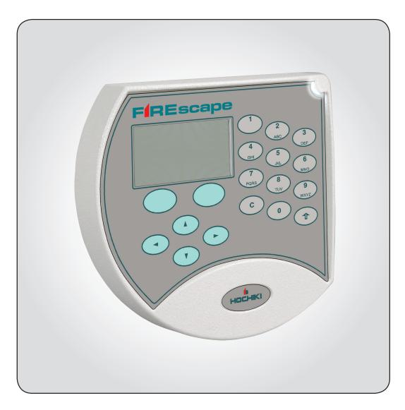
EL-KP is an emergency lighting control panel keypad for use with the EL-2 panel. The control panel is operated and interrogated through the compact backlit LCD graphical display of the keypad, which can show system status of the lighting units including battery charge and LED faults. One EL-2 control panel can support a total of 8 EL-KP keypad units, with up to a max of 15 panels on one system.
